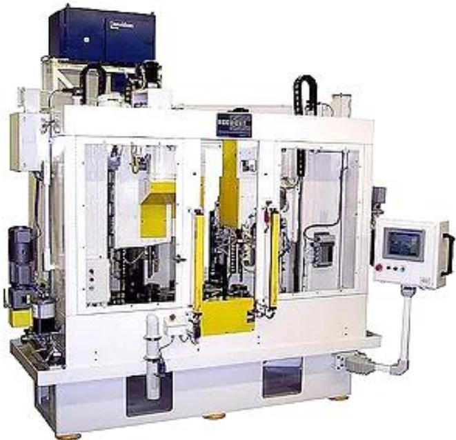
This machining operation will allow us to provide a part within one class (0.0001) thereby eliminating the need to classify valve bodies within 20 classes (0.002).
